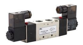
NITRA solenoid valve, 5-port (4-way), 2-position, double solenoid, (1) 3/8in female NPT inlet(s), (2) 3/8in female NPT outlet(s), (2) 1/4in female NPT exhaust(s), Cv=1.68, 120 VAC, 4.5VA, 11mm DIN style wiring plug.
