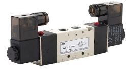
NITRA solenoid valve, 5-port (4-way), 2-position, double solenoid, (1) 1/4in female NPT inlet(s), (2) 1/4in female NPT outlet(s), (2) 1/4in female NPT exhaust(s), Cv=1.4, 120 VAC, 4.5VA, 11mm DIN style wiring plug.
