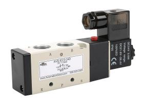
NITRA solenoid valve, 5-port (4-way), 2-position, single solenoid spring return, (1) 3/8in female NPT inlet(s), (2) 3/8in female NPT outlet(s), (2) 1/4in female NPT exhaust(s), Cv=1.68, 24 VDC, 3.0W, 11mm DIN style wiring plug.
