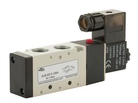
NITRA solenoid valve, 5-port (4-way), 2-position, single solenoid spring return, (1) 3/8in female NPT inlet(s), (2) 3/8in female NPT outlet(s), (2) 1/4in female NPT exhaust(s), Cv=1.68, 120 VAC, 4.5VA, 11mm DIN style wiring plug.
