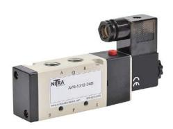
NITRA solenoid valve, 5-port (4-way), 2-position, single solenoid spring return, (1) 1/4in female NPT inlet(s), (2) 1/4in female NPT outlet(s), (2) 1/4in female NPT exhaust(s), Cv=1.4, 24 VDC, 3.0W, 11mm DIN style wiring plug.
