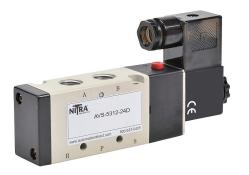
NITRA solenoid valve, 5-port (4-way), 2-position, single solenoid spring return, (1) 1/4in female NPT inlet(s), (2) 1/4in female NPT outlet(s), (2) 1/4in female NPT exhaust(s), Cv=1.4, 24 VDC, 3.0W, 11mm DIN style wiring plug.
