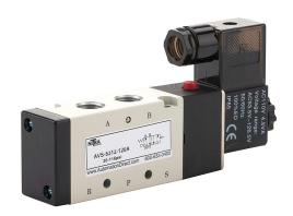
NITRA solenoid valve, 5-port (4-way), 2-position, single solenoid spring return, (1) 1/4in female NPT inlet(s), (2) 1/4in female NPT outlet(s), (2) 1/4in female NPT exhaust(s), Cv=1.4, 120 VAC, 4.5VA, 11mm DIN style wiring plug.
