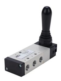
NITRA pneumatic manual valve, 5-port (4-way), 3-position, center exhaust, 90 deg hand lever, spring return, 1/8in female NPT inlet(s), 1/8in female NPT outlet(s), 1/8in female NPT exhaust(s), Cv=0.67, panel or surface mount.
