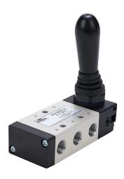
NITRA pneumatic manual valve, 5-port (4-way), 3-position, center exhaust, 90 deg hand lever, detented, 1/8in female NPT inlet(s), 1/8in female NPT outlet(s), 1/8in female NPT exhaust(s), Cv=0.67, panel or surface mount.
