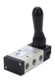
NITRA pneumatic manual valve, 5-port (4-way), 3-position, center closed, 90 deg hand lever, detented, 1/8in female NPT inlet(s), 1/8in female NPT outlet(s), 1/8in female NPT exhaust(s), Cv=0.67, panel or surface mount.
