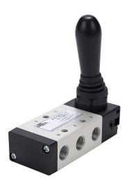
NITRA manual valve, 5-port (4-way), 3-position, center closed, handle, detented, 1/8in female NPT inlet(s), 1/8in female NPT outlet(s), 1/8in female NPT exhaust(s), Cv=0.67, panel or surface mount.
