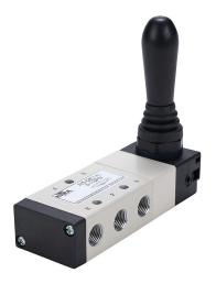
NITRA pneumatic manual valve, 5-port (4-way), 3-position, center closed, 90 deg hand lever, spring return, 1/8in female NPT inlet(s), 1/8in female NPT outlet(s), 1/8in female NPT exhaust(s), Cv=0.67, panel or surface mount.
