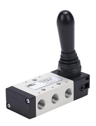
NITRA pneumatic manual valve, 5-port (4-way), 2-position, 90 deg hand lever, detented, 1/8in female NPT inlet(s), 1/8in female NPT outlet(s), Cv=0.78, panel or surface mount.
