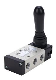
NITRA pneumatic manual valve, 5-port (4-way), 2-position, 90 deg hand lever, spring return, 1/8in female NPT inlet(s), 1/8in female NPT outlet(s), 1/8in female NPT exhaust(s), Cv=0.78, panel or surface mount.
