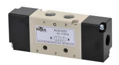
NITRA pilot valve, 5-port (4-way), 2-position, double air pilot, (1) 1/8in female NPT inlet(s), (2) 1/8in female NPT outlet(s), (2) 1/8in female NPT exhaust(s), Cv=0.78.
