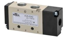
NITRA pilot valve, 5-port (4-way), 2-position, single air pilot spring return, (1) 1/4in female NPT inlet(s), (2) 1/4in female NPT outlet(s), (2) 1/8in female NPT exhaust(s), Cv=0.89.
