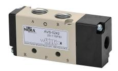
NITRA pilot valve, 5-port (4-way), 2-position, single air pilot spring return, (1) 1/4in female NPT inlet(s), (2) 1/4in female NPT outlet(s), (2) 1/8in female NPT exhaust(s), Cv=0.89.
