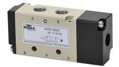
NITRA pilot valve, 5-port (4-way), 2-position, single air pilot spring return, (1) 1/8in female NPT inlet(s), (2) 1/8in female NPT outlet(s), (2) 1/8in female NPT exhaust(s), Cv=0.78.
