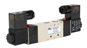
NITRA solenoid valve, 5-port (4-way), 3-position, center exhaust, double solenoid, (1) 1/4in female NPT inlet(s), (2) 1/4in female NPT outlet(s), (2) 1/8in female NPT exhaust(s), Cv=0.67, 24 VDC, 3.0W, 11mm DIN style wiring plug.
