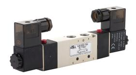
NITRA solenoid valve, 5-port (4-way), 3-position, center exhaust, double solenoid, (1) 1/4in female NPT inlet(s), (2) 1/4in female NPT outlet(s), (2) 1/8in female NPT exhaust(s), Cv=0.67, 120 VAC, 4.5VA, 11mm DIN style wiring plug.
