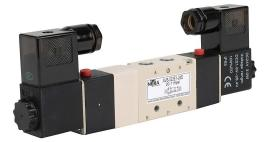
NITRA solenoid valve, 5-port (4-way), 3-position, center exhaust, double solenoid, (1) 1/8in female NPT inlet(s), (2) 1/8in female NPT outlet(s), (2) 1/8in female NPT exhaust(s), Cv=0.67, 24 VDC, 3.0W, 11mm DIN style wiring plug.
