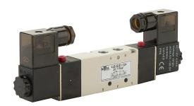
NITRA solenoid valve, 5-port (4-way), 3-position, center exhaust, double solenoid, (1) 1/8in female NPT inlet(s), (2) 1/8in female NPT outlet(s), (2) 1/8in female NPT exhaust(s), Cv=0.67, 120 VAC, 4.5VA, 11mm DIN style wiring plug.
