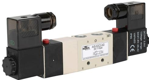
NITRA solenoid valve, 5-port (4-way), 3-position, center closed, double solenoid, (1) 1/4in female NPT inlet(s), (2) 1/4in female NPT outlet(s), (2) 1/8in female NPT exhaust(s), Cv=0.67, 24 VDC, 3.0W, 11mm DIN style wiring plug.
