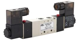
NITRA solenoid valve, 5-port (4-way), 3-position, center closed, double solenoid, (1) 1/4in female NPT inlet(s), (2) 1/4in female NPT outlet(s), (2) 1/8in female NPT exhaust(s), Cv=0.67, 120 VAC, 4.5VA, 11mm DIN style wiring plug.
