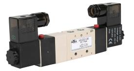
NITRA solenoid valve, 5-port (4-way), 3-position, center closed, double solenoid, (1) 1/8in female NPT inlet(s), (2) 1/8in female NPT outlet(s), (2) 1/8in female NPT exhaust(s), Cv=0.67, 24 VDC, 3.0W, 11mm DIN style wiring plug.
