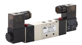
NITRA solenoid valve, 5-port (4-way), 3-position, center closed, double solenoid, (1) 1/8in female NPT inlet(s), (2) 1/8in female NPT outlet(s), (2) 1/8in female NPT exhaust(s), Cv=0.67, 120 VAC, 4.5VA, 11mm DIN style wiring plug.
