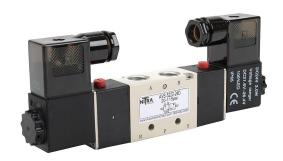
NITRA solenoid valve, 5-port (4-way), 2-position, double solenoid, (1) 1/4in female NPT inlet(s), (2) 1/4in female NPT outlet(s), (2) 1/8in female NPT exhaust(s), Cv=0.89, 24 VDC, 3.0W, 11mm DIN style wiring plug.
