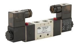
NITRA solenoid valve, 5-port (4-way), 2-position, double solenoid, (1) 1/4in female NPT inlet(s), (2) 1/4in female NPT outlet(s), (2) 1/8in female NPT exhaust(s), Cv=0.89, 120 VAC, 4.5VA, 11mm DIN style wiring plug.
