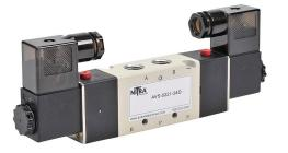
NITRA solenoid valve, 5-port (4-way), 2-position, double solenoid, (1) 1/8in female NPT inlet(s), (2) 1/8in female NPT outlet(s), (2) 1/8in female NPT exhaust(s), Cv=0.78, 24 VDC, 3.0W, 11mm DIN style wiring plug.
