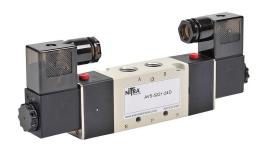
NITRA solenoid valve, 5-port (4-way), 2-position, double solenoid, (1) 1/8in female NPT inlet(s), (2) 1/8in female NPT outlet(s), (2) 1/8in female NPT exhaust(s), Cv=0.78, 24 VDC, 3.0W, 11mm DIN style wiring plug.
