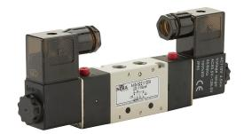
NITRA solenoid valve, 5-port (4-way), 2-position, double solenoid, (1) 1/8in female NPT inlet(s), (2) 1/8in female NPT outlet(s), (2) 1/8in female NPT exhaust(s), Cv=0.78, 120 VAC, 4.5VA, 11mm DIN style wiring plug.
