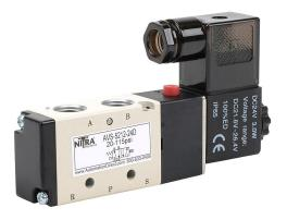
NITRA solenoid valve, 5-port (4-way), 2-position, single solenoid spring return, (1) 1/4in female NPT inlet(s), (2) 1/4in female NPT outlet(s), (2) 1/8in female NPT exhaust(s), Cv=0.89, 24 VDC, 3.0W, 11mm DIN style wiring plug.
