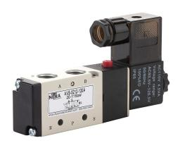
NITRA solenoid valve, 5-port (4-way), 2-position, single solenoid spring return, (1) 1/4in female NPT inlet(s), (2) 1/4in female NPT outlet(s), (2) 1/8in female NPT exhaust(s), Cv=0.89, 120 VAC, 4.5VA, 11mm DIN style wiring plug.
