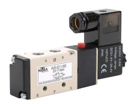
NITRA solenoid valve, 5-port (4-way), 2-position, single solenoid spring return, (1) 1/8in female NPT inlet(s), (2) 1/8in female NPT outlet(s), (2) 1/8in female NPT exhaust(s), Cv=0.78, 24 VDC, 3.0W, 11mm DIN style wiring plug.
