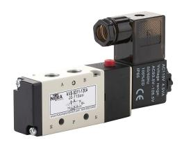
NITRA solenoid valve, 5-port (4-way), 2-position, single solenoid spring return, (1) 1/8in female NPT inlet(s), (2) 1/8in female NPT outlet(s), (2) 1/8in female NPT exhaust(s), Cv=0.78, 120 VAC, 4.5VA, 11mm DIN style wiring plug.
