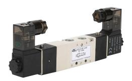
NITRA solenoid valve, 5-port (4-way), 3-position, center exhaust, double solenoid, (1) 1/8in female NPT inlet(s), (2) 1/8in female NPT outlet(s), (2) 1/8in female NPT exhaust(s), Cv=0.5, 24 VDC, 2.5W, 9.4mm DIN style wiring plug.
