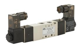
NITRA solenoid valve, 5-port (4-way), 3-position, center exhaust, double solenoid, (1) 1/8in female NPT inlet(s), (2) 1/8in female NPT outlet(s), (2) 1/8in female NPT exhaust(s), Cv=0.5, 120 VAC, 3.5VA, 9.4mm DIN style wiring plug.
