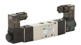
NITRA solenoid valve, 5-port (4-way), 3-position, center exhaust, double solenoid, (1) 1/8in female NPT inlet(s), (2) 1/8in female NPT outlet(s), (2) 1/8in female NPT exhaust(s), Cv=0.5, 120 VAC, 3.5VA, 9.4mm DIN style wiring plug.
