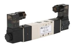
NITRA solenoid valve, 5-port (4-way), 3-position, center closed, double solenoid, (1) 1/8in female NPT inlet(s), (2) 1/8in female NPT outlet(s), (2) 1/8in female NPT exhaust(s), Cv=0.5, 24 VDC, 2.5W, 9.4mm DIN style wiring plug.
