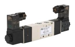
NITRA solenoid valve, 5-port (4-way), 3-position, center closed, double solenoid, (1) 1/8in female NPT inlet(s), (2) 1/8in female NPT outlet(s), (2) 1/8in female NPT exhaust(s), Cv=0.5, 24 VDC, 2.5W, 9.4mm DIN style wiring plug.
