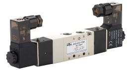
NITRA solenoid valve, 5-port (4-way), 3-position, center closed, double solenoid, (1) 1/8in female NPT inlet(s), (2) 1/8in female NPT outlet(s), (2) 1/8in female NPT exhaust(s), Cv=0.5, 120 VAC, 3.5VA, 9.4mm DIN style wiring plug.
