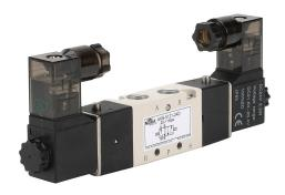
NITRA solenoid valve, 5-port (4-way), 2-position, double solenoid, (1) 1/8in female NPT inlet(s), (2) 1/8in female NPT outlet(s), (2) 1/8in female NPT exhaust(s), Cv=0.67, 24 VDC, 2.5W, 9.4mm DIN style wiring plug.
