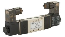
NITRA solenoid valve, 5-port (4-way), 2-position, double solenoid, (1) 1/8in female NPT inlet(s), (2) 1/8in female NPT outlet(s), (2) 1/8in female NPT exhaust(s), Cv=0.67, 120 VAC, 3.5VA, 9.4mm DIN style wiring plug.
