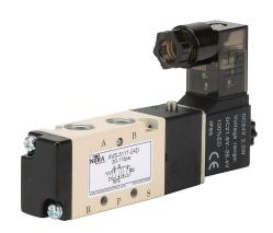
NITRA solenoid valve, 5-port (4-way), 2-position, single solenoid spring return, (1) 1/8in female NPT inlet(s), (2) 1/8in female NPT outlet(s), (2) 1/8in female NPT exhaust(s), Cv=0.67, 24 VDC, 2.5W, 9.4mm DIN style wiring plug.
