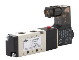
NITRA solenoid valve, 5-port (4-way), 2-position, single solenoid spring return, (1) 1/8in female NPT inlet(s), (2) 1/8in female NPT outlet(s), (2) 1/8in female NPT exhaust(s), Cv=0.67, 120 VAC, 3.5VA, 9.4mm DIN style wiring plug.
