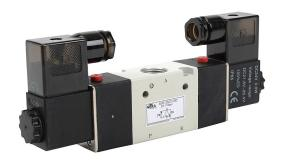
NITRA solenoid valve, 3-port (3-way), 2-position, double solenoid, (1) 3/8in female NPT inlet(s), (1) 3/8in female NPT outlet(s), (1) 3/8in female NPT exhaust(s), Cv=1.67, 24 VDC, 3.0W, 11mm DIN style wiring plug.
