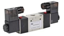
NITRA solenoid valve, 3-port (3-way), 2-position, double solenoid, (1) 1/4in female NPT inlet(s), (1) 1/4in female NPT outlet(s), (1) 1/4in female NPT exhaust(s), Cv=1.39, 24 VDC, 3.0W, 11mm DIN style wiring plug.
