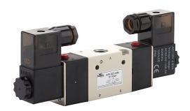
NITRA solenoid valve, 3-port (3-way), 2-position, double solenoid, (1) 1/4in female NPT inlet(s), (1) 1/4in female NPT outlet(s), (1) 1/4in female NPT exhaust(s), Cv=1.39, 120 VAC, 4.5VA, 11mm DIN style wiring plug.
