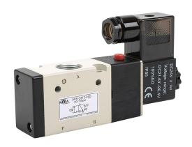
NITRA solenoid valve, 3-port (3-way), 2-position, N.C., single solenoid spring return, (1) 3/8in female NPT inlet(s), (1) 3/8in female NPT outlet(s), (1) 3/8in female NPT exhaust(s), Cv=1.67, 24 VDC, 3.0W, 11mm DIN style wiring plug.
