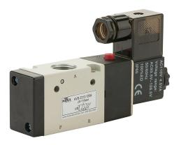
NITRA solenoid valve, 3-port (3-way), 2-position, N.C., single solenoid spring return, (1) 3/8in female NPT inlet(s), (1) 3/8in female NPT outlet(s), (1) 3/8in female NPT exhaust(s), Cv=1.67, 120 VAC, 4.5VA, 11mm DIN style wiring plug.
