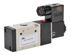
NITRA solenoid valve, 3-port (3-way), 2-position, N.C., single solenoid spring return, (1) 1/4in female NPT inlet(s), (1) 1/4in female NPT outlet(s), (1) 1/4in female NPT exhaust(s), Cv=1.39, 24 VDC, 3.0W, 11mm DIN style wiring plug.
