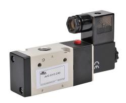
NITRA solenoid valve, 3-port (3-way), 2-position, N.C., single solenoid spring return, (1) 1/4in female NPT inlet(s), (1) 1/4in female NPT outlet(s), (1) 1/4in female NPT exhaust(s), Cv=1.39, 24 VDC, 3.0W, 11mm DIN style wiring plug.
