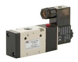
NITRA solenoid valve, 3-port (3-way), 2-position, N.C., single solenoid spring return, (1) 1/4in female NPT inlet(s), (1) 1/4in female NPT outlet(s), (1) 1/4in female NPT exhaust(s), Cv=1.39, 120 VAC, 4.5VA, 11mm DIN style wiring plug.
