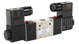
NITRA solenoid valve, 3-port (3-way), 2-position, double solenoid, (1) 1/4in female NPT inlet(s), (1) 1/4in female NPT outlet(s), (1) 1/4in female NPT exhaust(s), Cv=0.89, 24 VDC, 3.0W, 11mm DIN style wiring plug.
