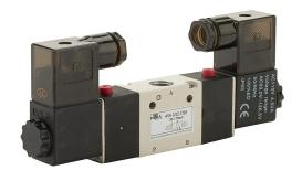
NITRA solenoid valve, 3-port (3-way), 2-position, double solenoid, (1) 1/4in female NPT inlet(s), (1) 1/4in female NPT outlet(s), (1) 1/4in female NPT exhaust(s), Cv=0.89, 120 VAC, 4.5VA, 11mm DIN style wiring plug.
