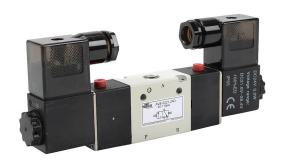
NITRA solenoid valve, 3-port (3-way), 2-position, double solenoid, (1) 1/8in female NPT inlet(s), (1) 1/8in female NPT outlet(s), (1) 1/8in female NPT exhaust(s), Cv=0.78, 24 VDC, 3.0W, 11mm DIN style wiring plug.
