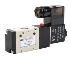
NITRA solenoid valve, 3-port (3-way), 2-position, N.C., single solenoid spring return, (1) 1/4in female NPT inlet(s), (1) 1/4in female NPT outlet(s), (1) 1/4in female NPT exhaust(s), Cv=0.89, 24 VDC, 3.0W, 11mm DIN style wiring plug.
